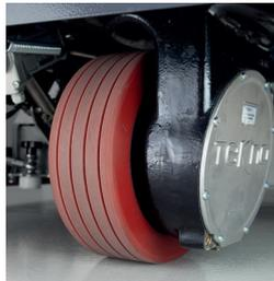
Powerful and reliable, the traction motor is vertically installed in the front part of the machine. The front wheel is driven via a gear box which is lubricated and sealed to protect it against impact, dirt, and humidity.
