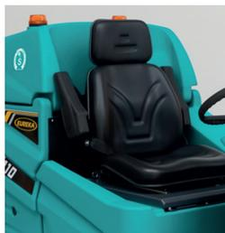
The operator's seat is equipped with weight sensors and a seat belt, it is also possible to cut off power in an emergency or during maintenance operations, guaranteeing maximum protection and safety to operators and mechanics.
