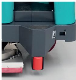
The robust frame realized in thick steel provides protection to both the operator and the internal parts of the machine. The optional overhead guard can be fitted to the E110-D for added safety.
