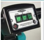
For added safety the E46 has a starter key. The brush motor and electric circuit are protected by a resettable fuse, which interrupts the power supply should an anomaly occur.
